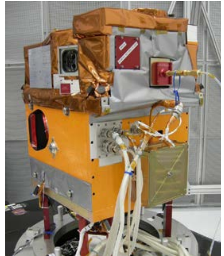
The dragNET de-orbit system fully stowed and integrated on the STPSat-3 spacecraft.
